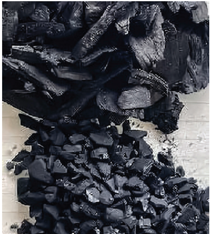
Figure 19: A closeup comparative view of the biochar and the re-activated carbon. The re-activated carbon is smaller and harder, the biochar is larger and softer. Both activated materials are used as part of a broad-spectrum affinity.
