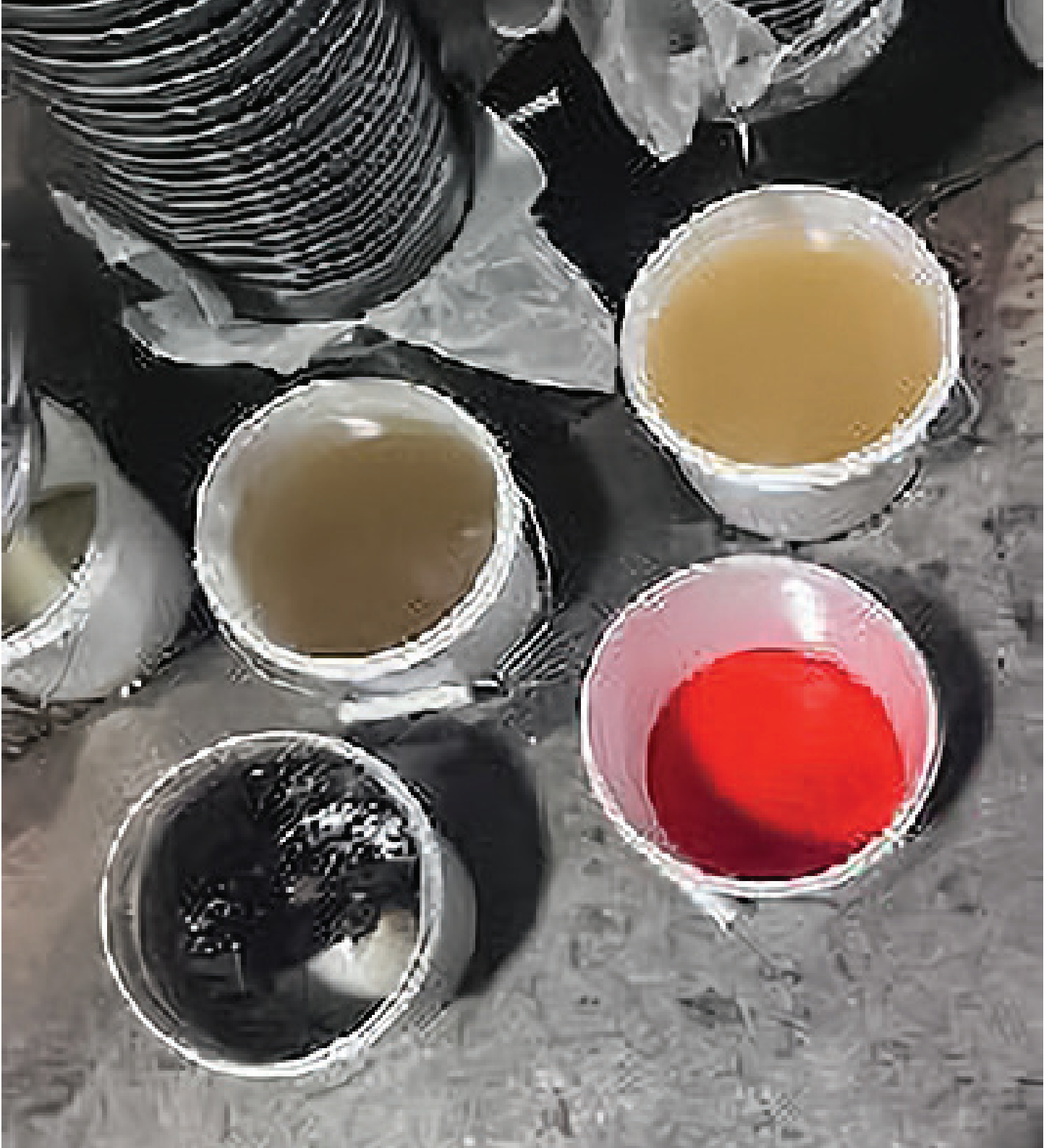
Figure 30: For motor oil, diesel, and gasoline the 3 liters per tube were mixed and poured separately so each tube would get the right amount of pollutant in the water. This gave rise to this picture. On the right is motor oil and water ready for the second tube pour, and the bucket directly above it is the output from the first tube pour moments before – almost no oil showing. More interesting was the bucket to the right – red dye diesel set up for the second tube pour (water not yet added). Directly above it is the output from the first tube pour moments before – almost no red dye showing. We observed throughout the 20 simulated rain events – almost no hydrocarbons getting through.
