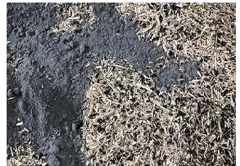
Figure 6: CSA being added to Char21 SW
