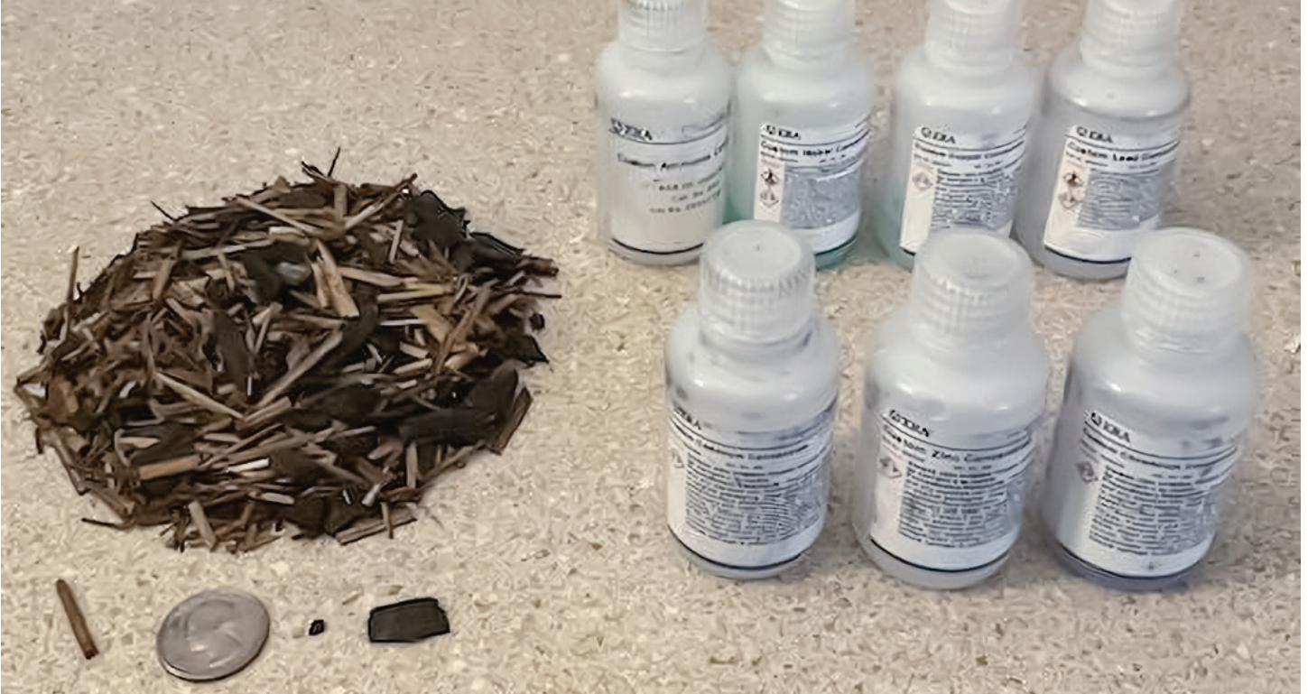
Figure 34: Dried sample of Char21™ SW removed from the vertical tube after 3 months and 20 rain events. Also shown are the 50 ml pollutant bottles used from ERA Lab. Also shown is a piece of switchgrass, a quarter, a piece of re-activated carbon, and a chunk of biochar.
