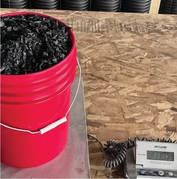
Figure 20: Measuring bulk density of the biochar. Since bucket weighs 2.2 lbs., the sampled biochar is about 9.5 lbs. per 5-gallon bucket. 41 buckets per cubic yard calculates to 389 lbs. per cubic yard.
