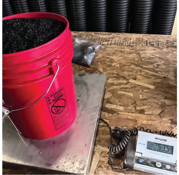
Figure 21: Measuring the bulk density of the re-activated carbon. Removing the bucket weight leaves about 23 lbs. but the bucket is slightly underfilled. Filled we estimate the 5-gallon bucket at 24.5 lbs. of re-activated carbon or about 1,000 lbs. per cubic yard.
