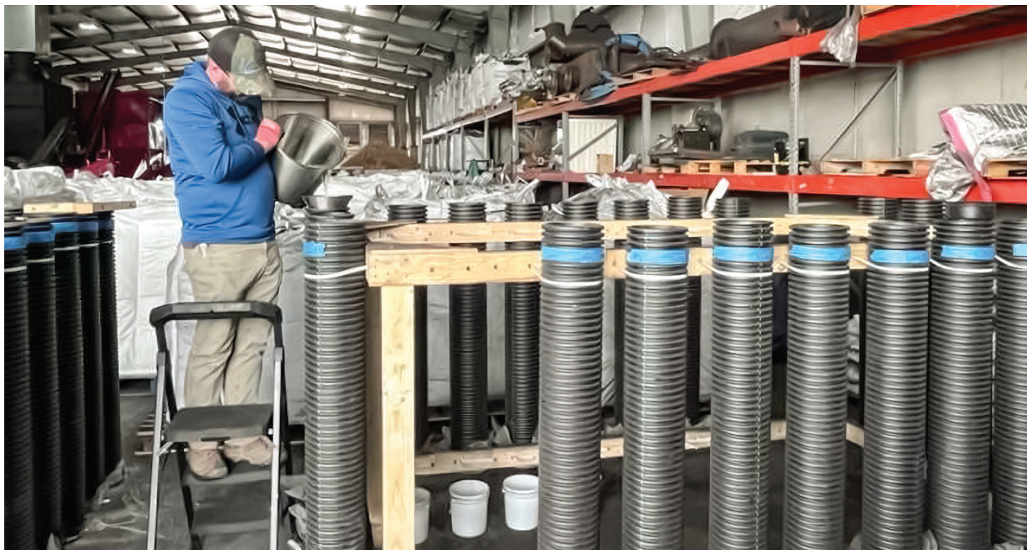
Figure 28: Another picture of lab tech pouring pollutant water. Notice that all vertical tubes in the test were labeled with blue painter's tape. Also notice the small white collection buckets at bottom of vertical flow tubes. Pouring the water into each tube took about 30 seconds. Early on in the test, the observed vertical flow time before water came out the bottom was about 30 seconds. This increased over time to about 40-45 seconds. We believed this was caused by the wetted filter media compressing over time.
