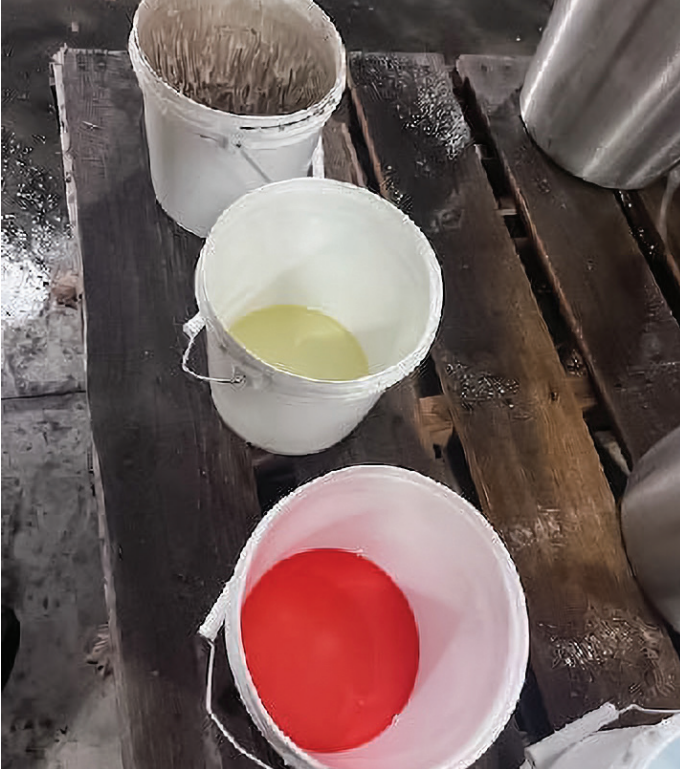
Figure 24: Motor oil, gasoline, and red-die diesel being measured out before being added to water.
