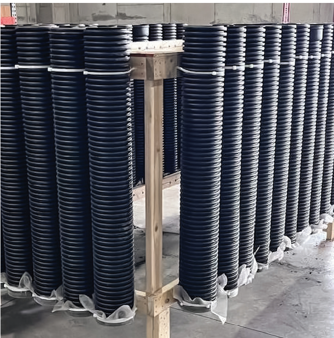
Figure 22: The vertical flow tubes. 48-inch long and 6-inch diameter N-12 smooth wall inside. Tube is filled with 36-inches of lightly compacted Char21™ SW with 12-inches open at top. A plastic mesh screen is zip-tied across the bottom of tube to allow water flow through but not Char21™ SW.
