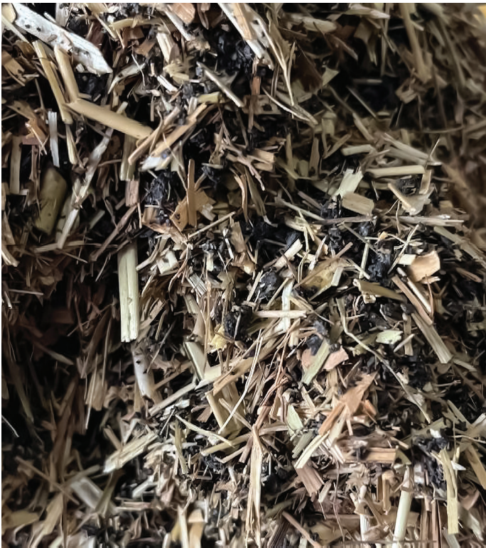
Figure 18: Closeup of blend – switchgrass, biochar, re-activated carbon, and CSA.
