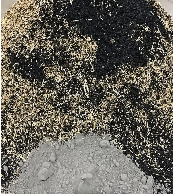
Figure 16: Re-activated carbon and CSA added before blending.
