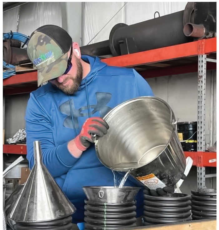
Figure 27: Lab tech pouring polluted water into top of vertical flow tube using stainless-steel bucket and stainless-steel funnel.
