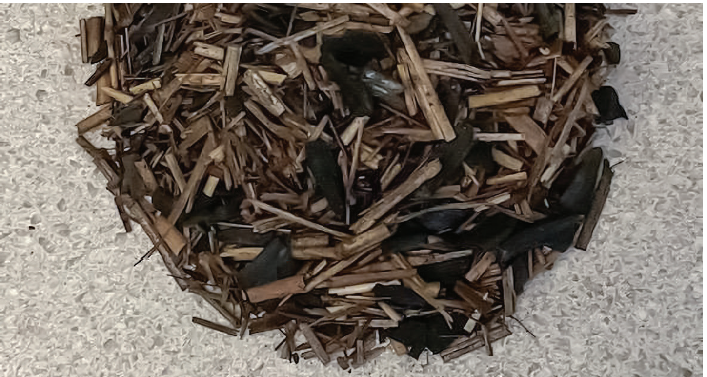
Figure 35: Same as Figure 34. The filter media is quite dark, but nothing is falling apart. Our observation is the media pollution affinity has not begun to diminish.
