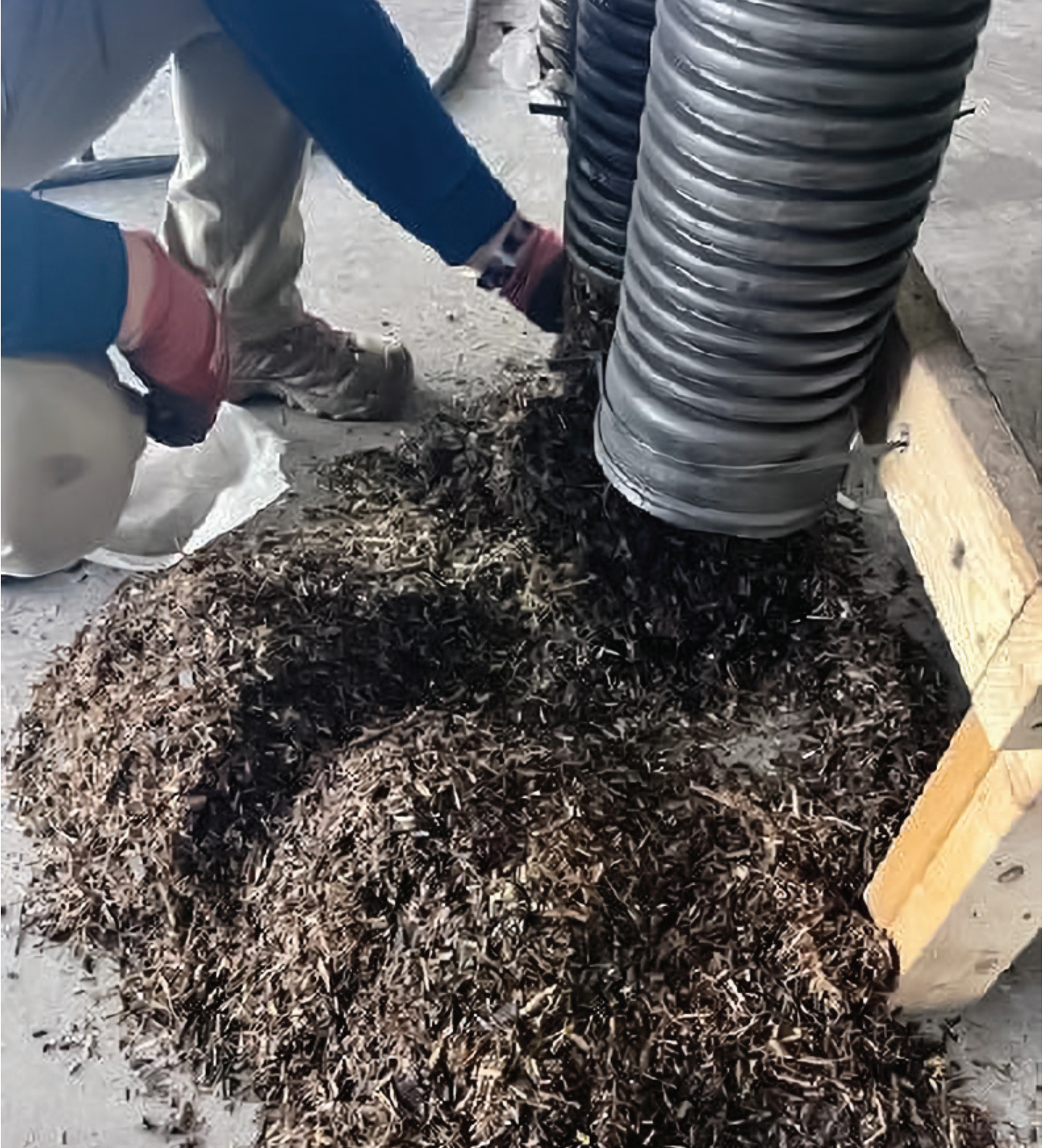
Figure 33: Picture of Char21™ SW fill removed from a vertical tube after the 3 months and 20 rain events. Notice the dark color. We think the switchgrass is beginning to decay in the vertical tube and contributed to the increase of pollutant affinity we observed.
