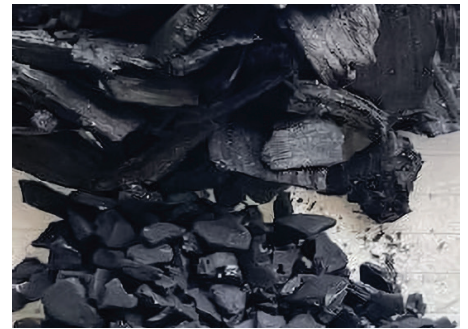
Figure 5: Large chunk biochar (top) next to re-activated carbon (bottom) in Char21 SW
