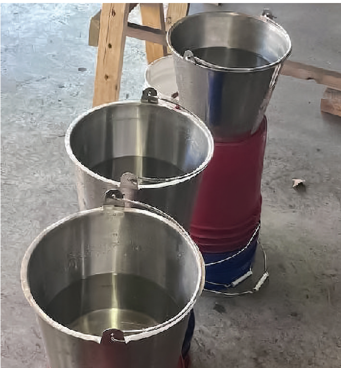
Figure 26: Three 6-liter samples ready to pour. For each pollutant, 2 tubes were set up with 3 liters being poured through each one. On the sample collection days, a small input sample was taken before pouring with the remainder being split between the two tubes. Output water from the two tubes was combined and a sample for the lab was collected.
