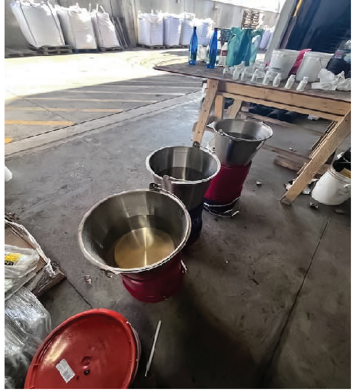
Figure 25: Stainless steel buckets were used to prepare 6 liters of polluted water per pollutant. The 50ml bottles from ERA Labs hold the pollutants. Buckets and funnels were rinsed between each pour.
