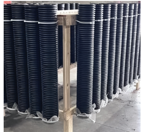
Figure 7: 6-inch diameter, 48-inch tall pipes filled with Char21 SW, with a mesh screen securing the media. Polluted water was poured in from the top, and filtered water exited the bottom. Two pipes were used per pollutant.
