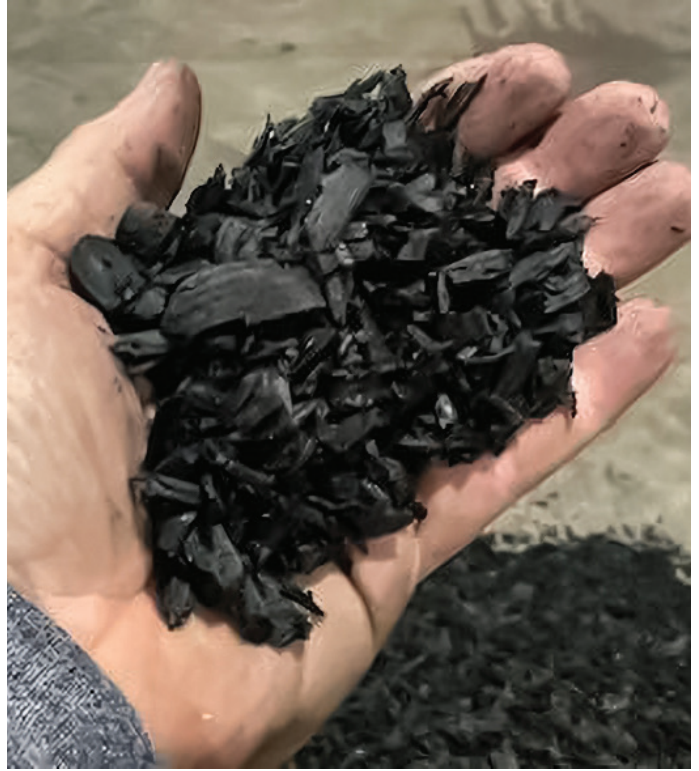
Figure 13: Large chunk hardwood biochar with +80% carbon content.
